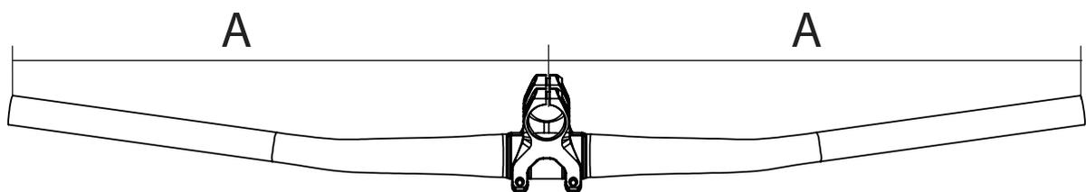
3. Tighten handlebar clamping bolts (M5x15) slightly.
